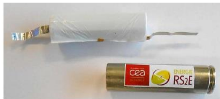
First 18650 Na-ion battery (1 Ah) made at CEA Grenoble
